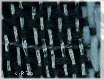
Cut protection fabric with cut detection
