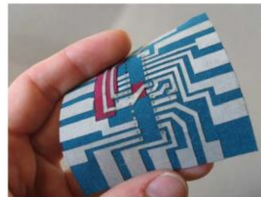
Textile circuit with heat pressed conductive fabric [6]
