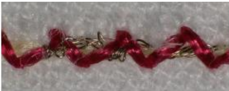
Torn Litz wires [19]
