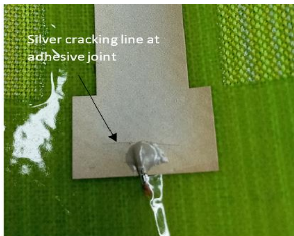
Failure at wire adhesive joints
