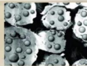
Outlast Thermo-molecules locked into the textile fiber
